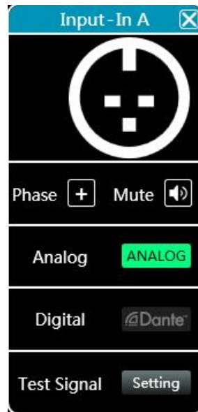
Figure 7.1 Channel input module
